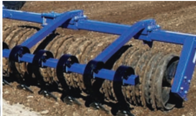
Mounted with hydraulically adjustable cracker board.
