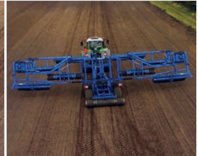
2. Side sections are folded out and lowered to the ground.
