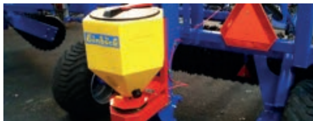
Granulate distributor for slug control.
