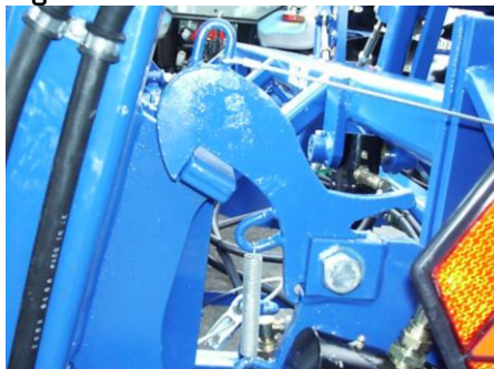
Transport lock on the packer roller
