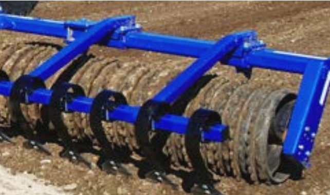
Mounted with hydraulically adjustable cracker board.
