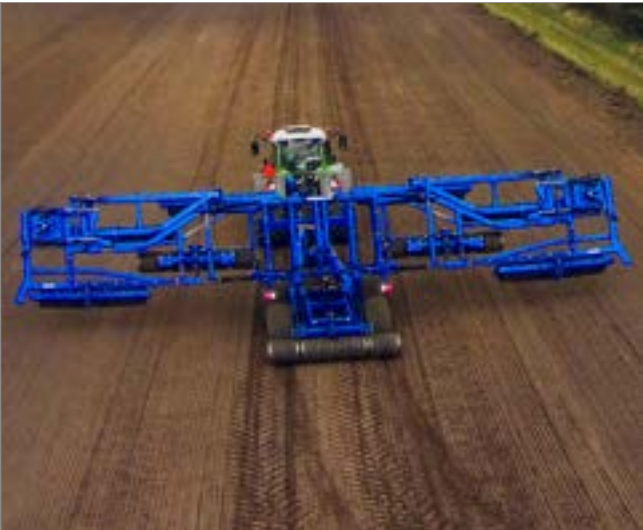
2. Side sections are folded out and lowered to the ground.
