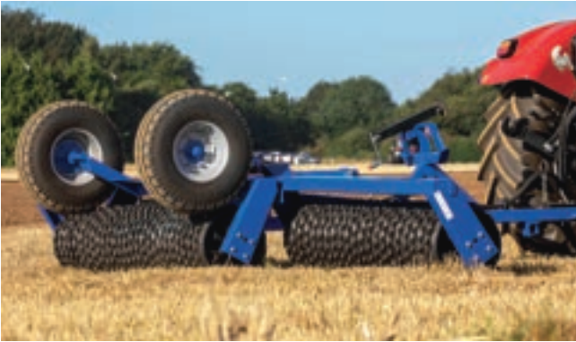
3. The roller sections are lowered to the working position and the wheels are automatically raised.
