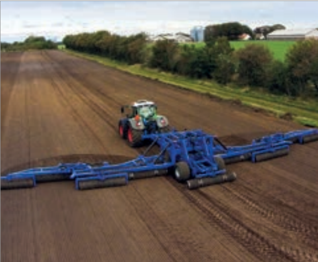
4. When the roller sections are in the working position, the 2 hydraulic weight distribution systems are at the correct working pressure and in the floating position, the wheels are automatically raised free of the ground.
