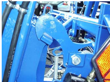
Transport lock on the packer roller
