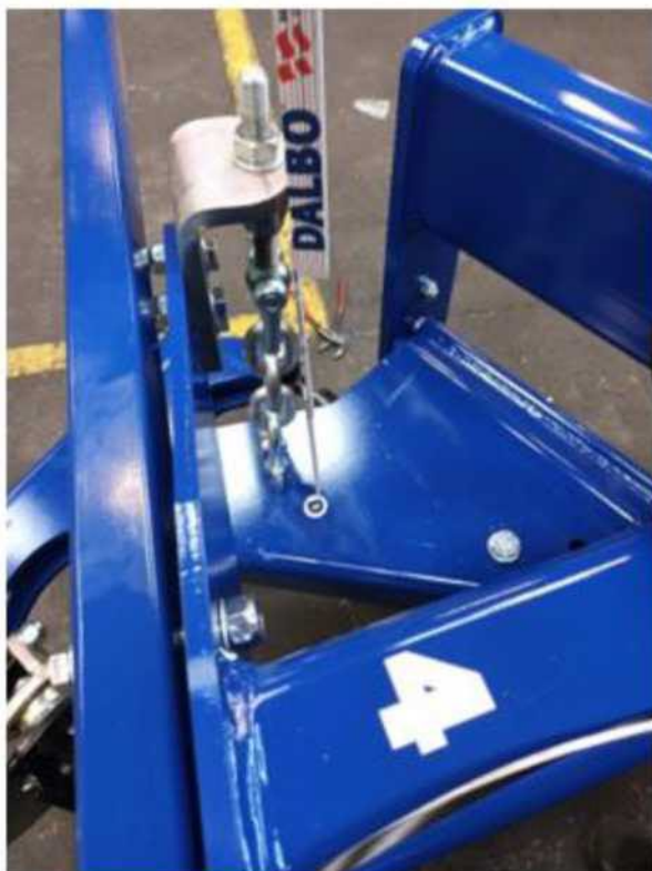
Spindle length support wheel C-C = 505 mm
