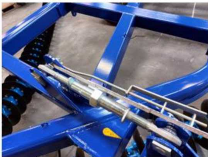
Spindle length support wheel C-C = 505 mm
