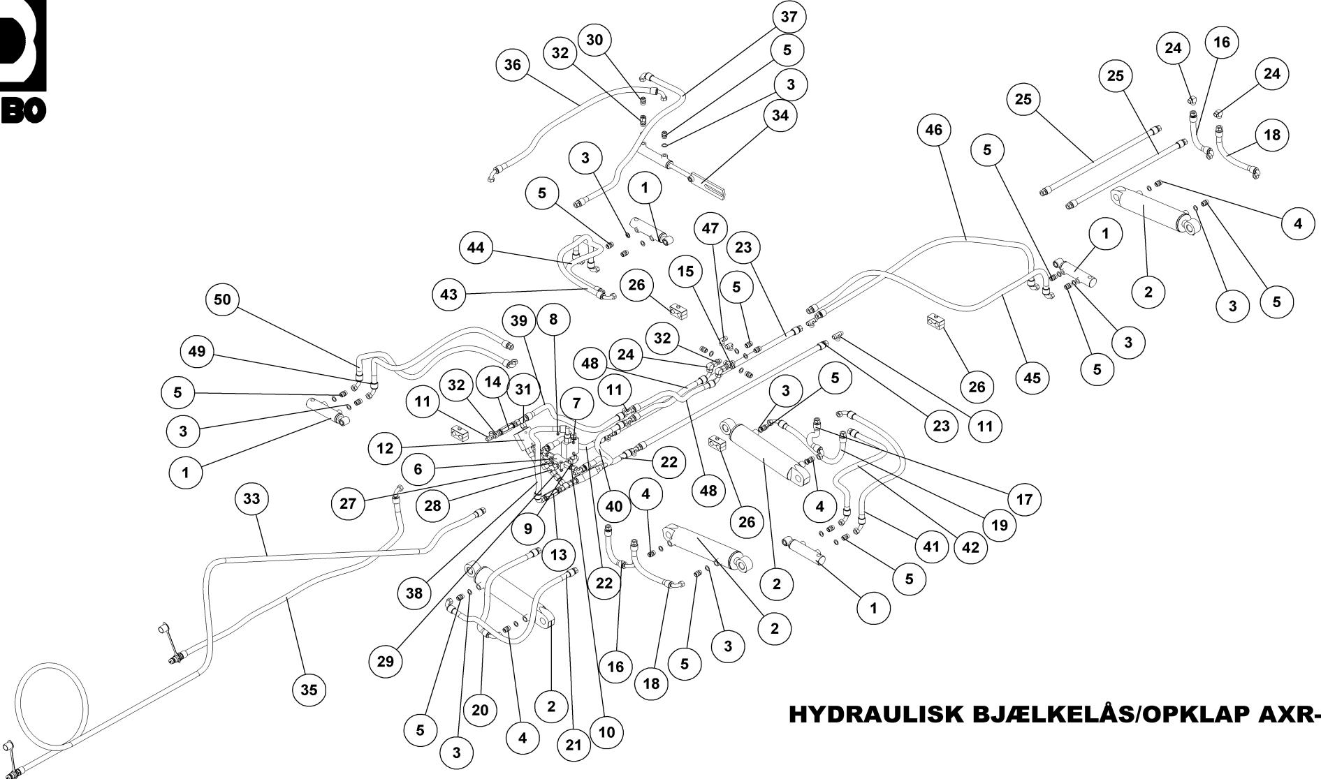
**HYDRAULISK BJÆLKELÅS/OPKLAP AXR-H**
